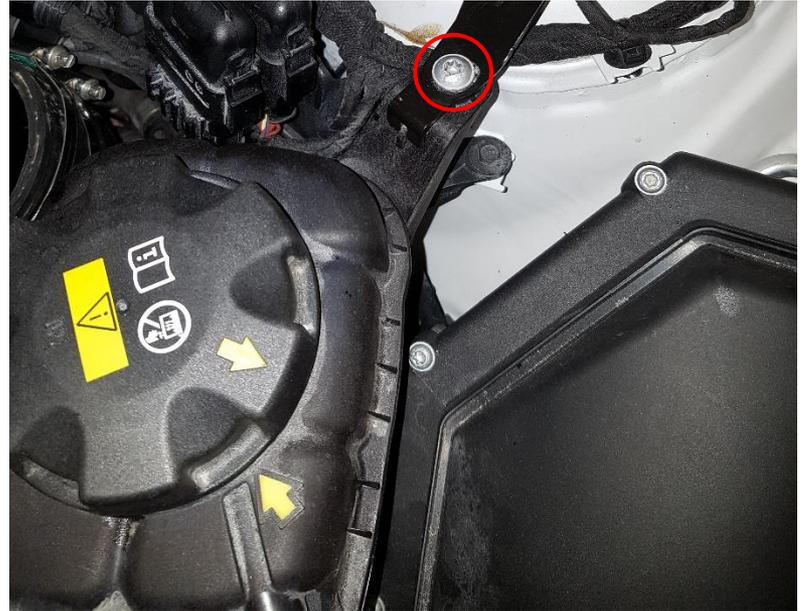
8. Use a flat screwdriver and gently pry the white tab up from its groove then use your fingers to pull the white plastic locking strip out. Remove 1x 6mm hose clamp located on the intercooler hose. Remove the plastic intercooler outlet pipe. Gently remove the O-rings from the OEM pipe and install them in the do88 intercooler outlet pipe. (You can use a little bit of engine oil on the o-ring for easier installation)
