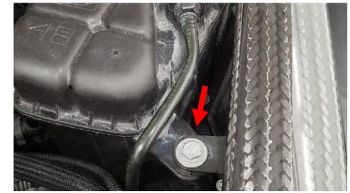
5. On the Coolant reservoir you'll find a plastic line. Loosen the clip for the plastic coolant line and separate from reservoir, use the included silicone caps to plug both connections.
