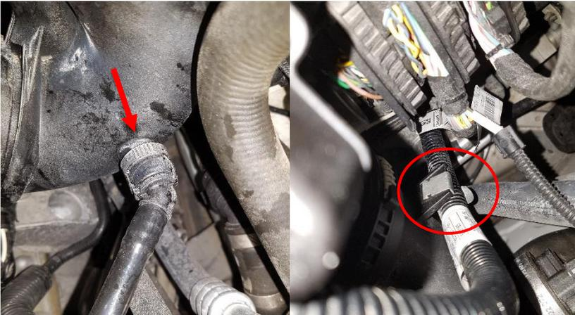
6. Remove 1x Torx T30, which will make the coolant reservoir able to move, strap it to a safe place, be careful of the connector and the coolant hose underneath.
