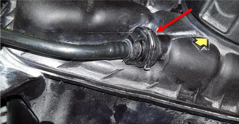
7. Disconnect the plastic hose and the cable secured on the intercooler outlet pipe. Secure the cable with the included zip tie.
