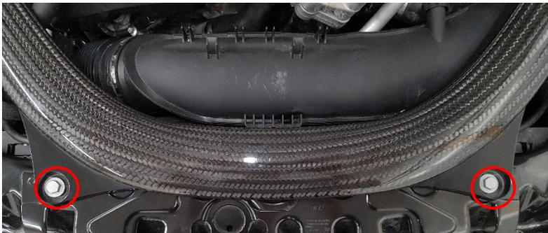
4. Remove 1x hex 10mm screw from bracket to coolant reservoir and remove the carbon fiber Strut brace from the vehicle.
