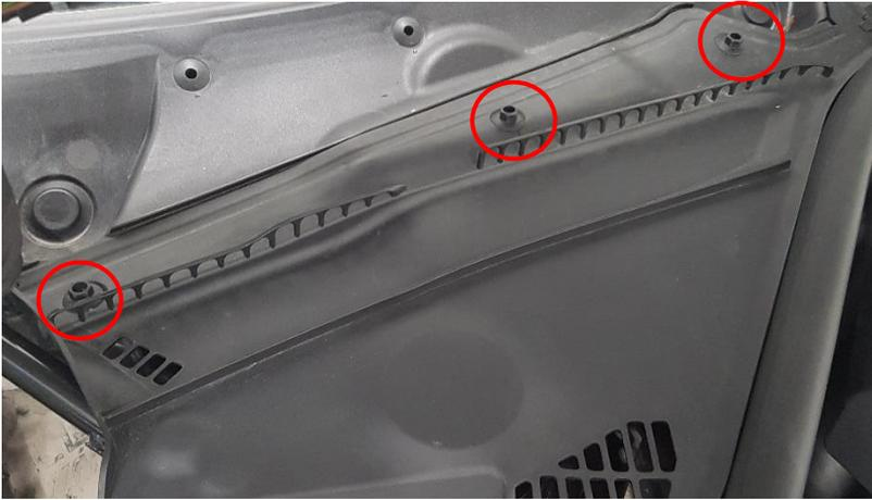
2. Remove this plastic clip with the help of a flathead screwdriver on both sides. Remove plastic covers.
