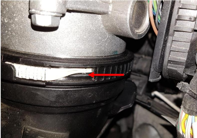
10. Use the included hose clamp to secure the do88 hose to the intercooler outlet pipe and intercooler.
