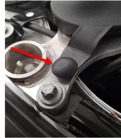
3. Remove 8x hex 13mm screws to the carbon fiber Strut brace, mounted across the engine.
