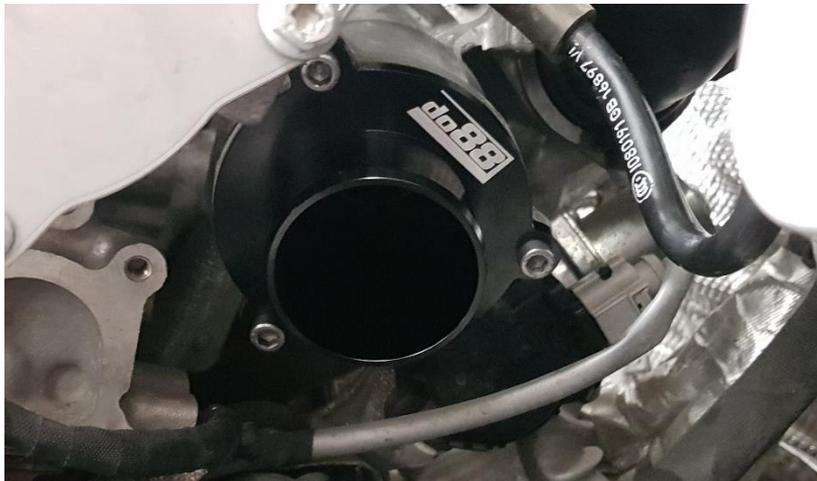
7. Install the included silicone hose and hose clamps in-between the turbo muffler delete and the intercooler pipe. Install all other parts in reverse order.
