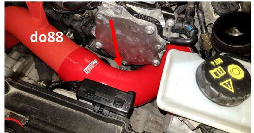
4. Remove 3x Allen screw 5mm.
