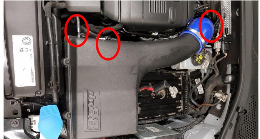
3. If you have OEM intercooler pipes: Loosen 1x Torx T30 screw at the pressure pipe bracket and remove the hose at the turbo outlet. Also disconnect the small plastic box from it bracket on the battery tray. Gently pull away the pipe now to make space at the turbo outlet.
